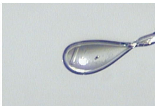
Figure 2 The endonuclease crystal used for data collection is shown mounted in a nylon loop. The longest dimension was measured to be 0.1 mm.
